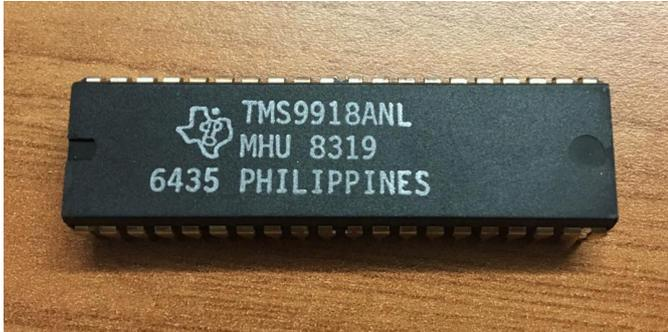
Figura 2: TMS9918A Video Display Processor
