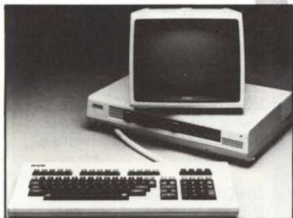
EPSON QX 10: personal computer, struttura a 8 microprocessori, 192 KBytes RAM min., 2 floppy da 320 KBytes, CP/M....
