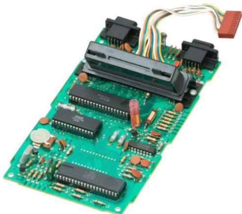
**Fig. 9 - the motherboard of the first version of the console. From above, the 3 main chips are: the MOS 6532 RIOT, the MOS 6507 CPU, and the Atari TIA (source: Wikimedia - author: Evan-Amos)**
