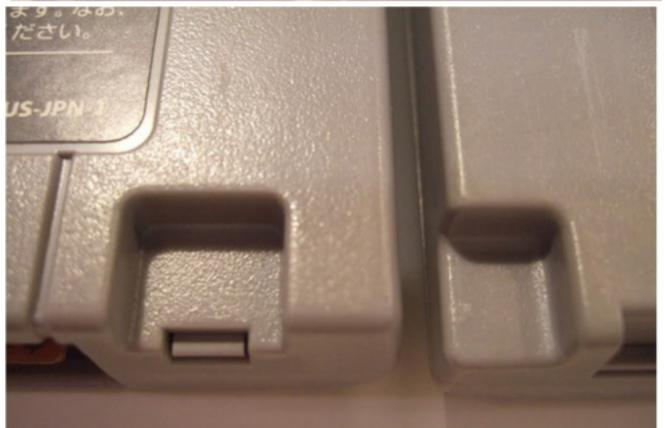
In order to get them in, a modification has to be made to the case by removing the tabs in the cartridge slot:
