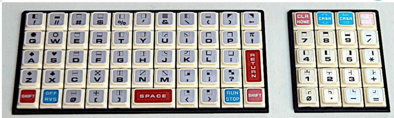
**Fig. 5 - The small keyboard with rubber keys of the early PETs**
