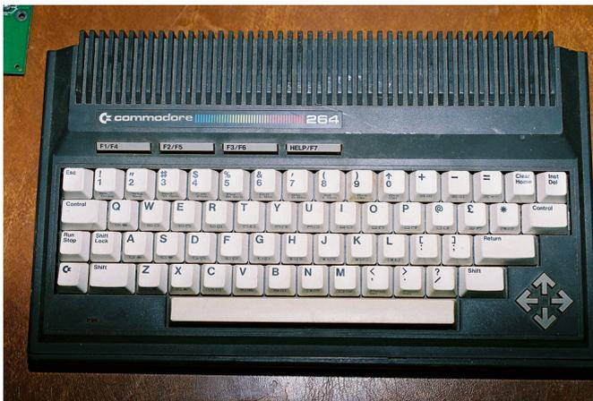
**Fig.1 - Commodore 264 prototype (photo by Babylon4 - source Mediawiki Commons)**
