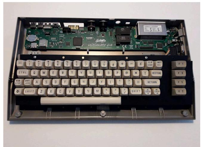
The Ultimate 64 installed in a Commodore 64 case
